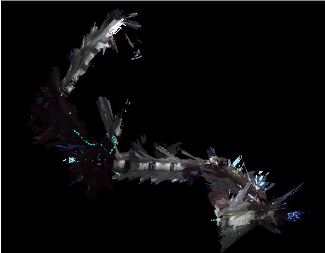
Fig. 3: RTAB-Map with failed loop closure
